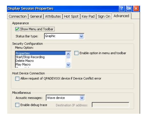
Appearance - option allows to show menu and toolbar or hide it. Use the drop down Status Bar type: to change the status bar.
