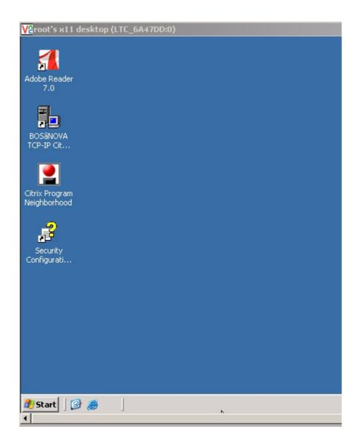
Maximized mode maximizes the RDP desktop but leaves the thin client toolbar visible underneath it.
