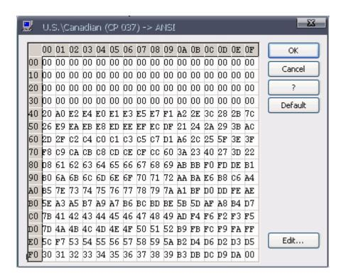
Code page is the traditional IBM term used for a specific character encoding table: a mapping in which a sequence of bits, usually a single octet representing integer values 0 through 255, is associated with a specific character.
