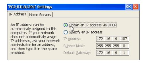
If you do not have a DHCP server on the network, the IP address and gateway must be set manually.
