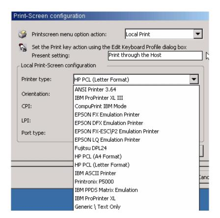
Printer type is limited to built in drivers, select the closest match. If in doubt, try Generic/Text Only or use Host Print Transform.
