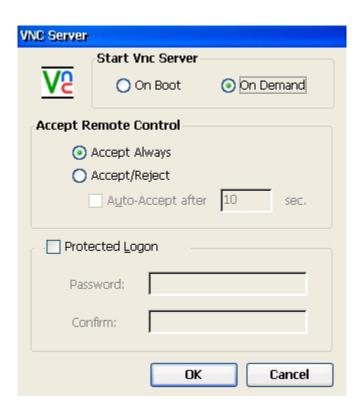
A password can be assigned to the unit by selecting Protected Logon and completing the password information. A warning message will be presented on the screen to make the user aware the unit is being shadowed.
