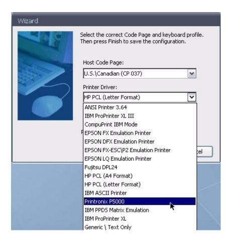
If unsure of the printer driver, try Generic\Text Only and/or use Host Print Transform in the Advanced tab.
