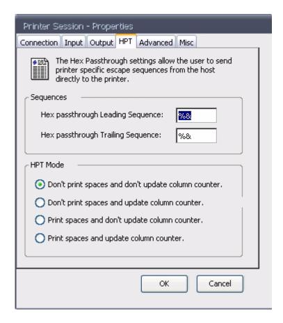
Some AS400 applications send "raw" sequences of commands to the printer - for instance to create custom overlays when using PCL. These commands should not be interpreted by the printer engine and are called hex passthru sequences. They are usually delimited by special characters so the printer engine can pass the data directly to the printer.
