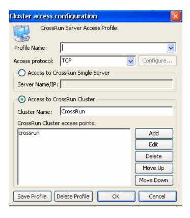
The Access Profiles section allows you to define a profile for accessing a CrossRun Server. To Access to CrossRun Server enter the Server Name/IP.
