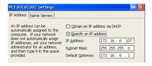
Name Servers tab allows for setting the DNS server to enable the browser to resolve host addresses. This most likely would be used only when you set the IP address manually.
