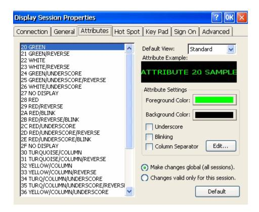
To change the column separator character select the Edit option to the right of the Column Separator.
