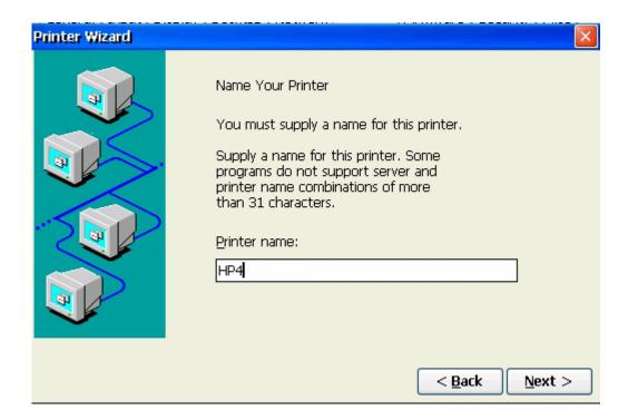
The WTC only supports SAMBA shared printers and needs a name such as \\PCNAME\printersharename. If trying to connect to a network printer put it on a server and share it and then the WTC can connect to it..
