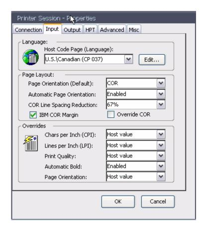
Computer output reduction (COR) automatically takes standard reports on computer paper and reduces them to fit on 8-1/2 by 11 inch paper. COR is designed to handle reports created at 66 lines per page and 132 print positions per line.
