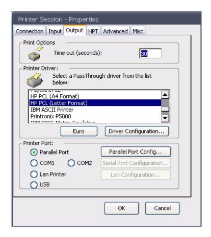
The timeout is the time that is elapsed before we notify the host that the printer is offline and/or unreachable.
