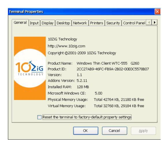
Checking the **Restore the terminal parameters to factory default** will reset all terminal parameters to the default state. Upon rebooting the terminal the Terminal Configuration Setup Wizard will appear. Factory defaults can also be reset from the remote terminal manager by right clicking on the unit and selecting Special Functions - Factory Default.
